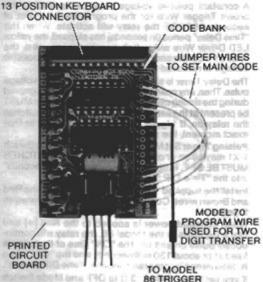
Example: If the Corby Key Main Code is 4-3-2-1-#, touching buttons 4 and 6 produces a positive voltage at the "Code Bank" (socket #6) which will trigger the Model 86. The voltage will remain on the Model 70 ProgramWire as long as the two buttons remain touched. This feature is available 24 hours a day.
